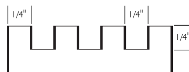
1/4" x 1/4" x 1/4" Square Notch > 1/2" Flat Milled Solid & Shorts or Plywood Coverage: 35 ft 2 /Gallon
